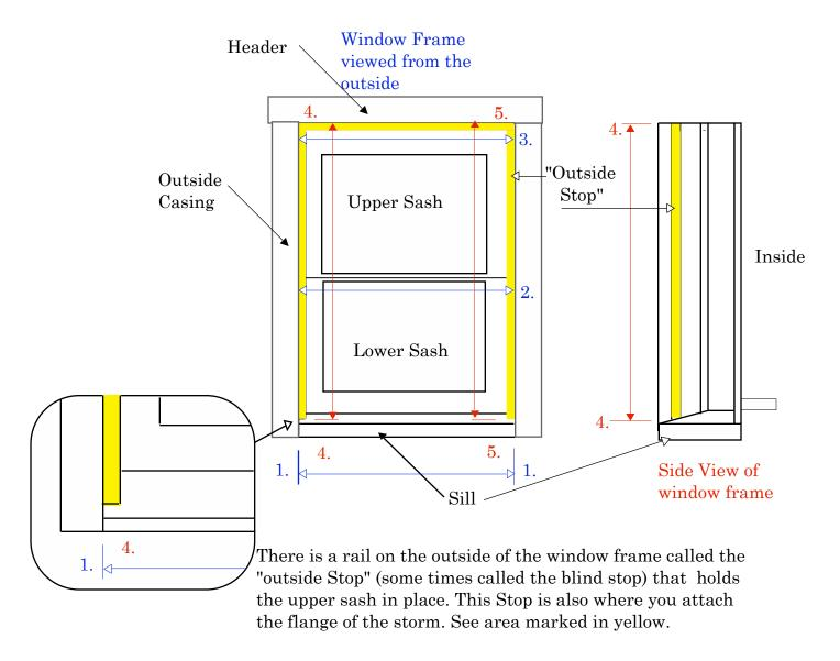
See Installing Vinyl Storm Windows Adv# 1. Measure the width of the window frame at three places 1,2,3, and the height in two places 4,5. This is called the window opening size.
